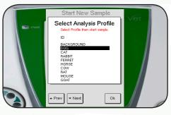
**12 different Species Profiles** 12 analysis profiles come pre-installed and new profiles can easily be added in the instrument.
