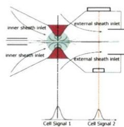
**Dual Sheath Flow Cell System and Intelligent Sample Treatment System**
