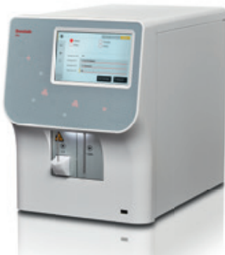
Swelab Alfa Plus Basic – even the basic model includes shear-valve technology.
