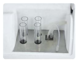
CliniQuant<sup>™</sup> has in-built incubator slots that provide accurate temperature for reagents and reaction mixtures thus ensuring optimal reaction with sample.
